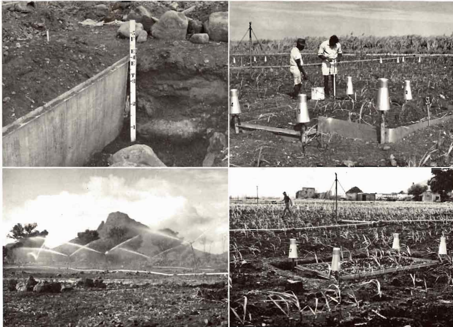
Lysimeter experiment at Palmyre
