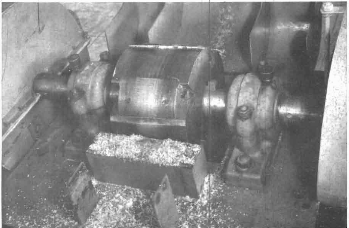
Fig. 40. Above : Cane chopper and Waring blenders, used for cane analysis from experimental plots. Below : Close-up of cane chopper (hood removed) showing chipped cane.
