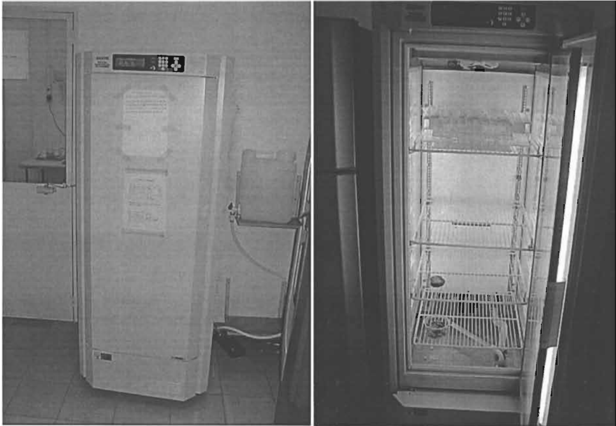
Figure 15 :Chambre climatique, 0 ... 50 °C, 294 l/MLR-352, MLR-352H-SANYO
