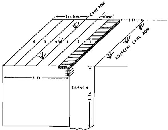
Fig. 15. Illustration of the digging procedure.
