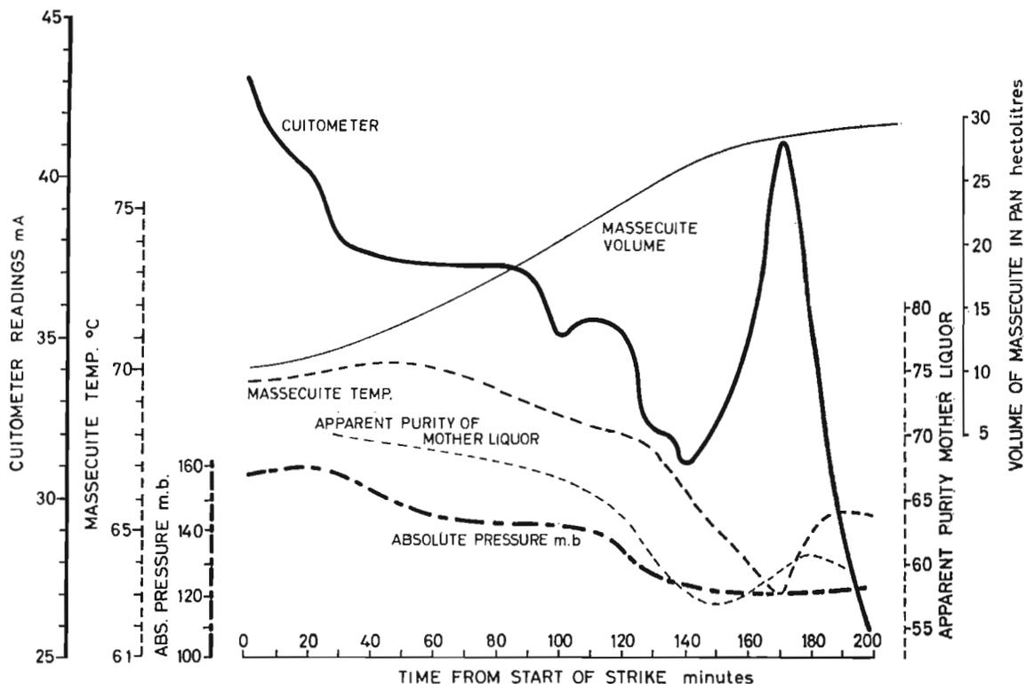
Fig. 15. Evolution of main parameters during a high grade strike.
