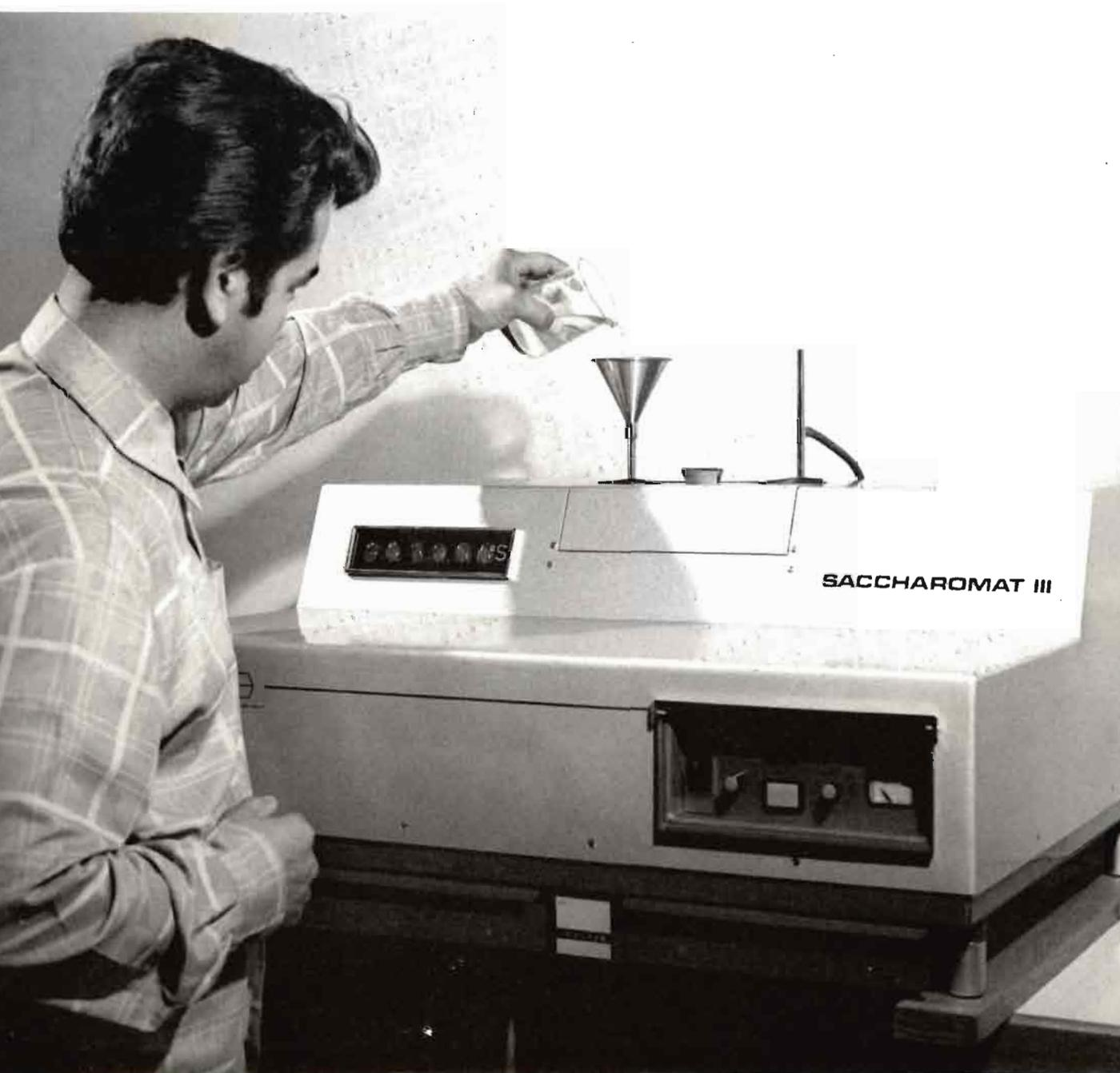
Plate VI. The Schmidt and Haensch Automatic Polarimeter.
