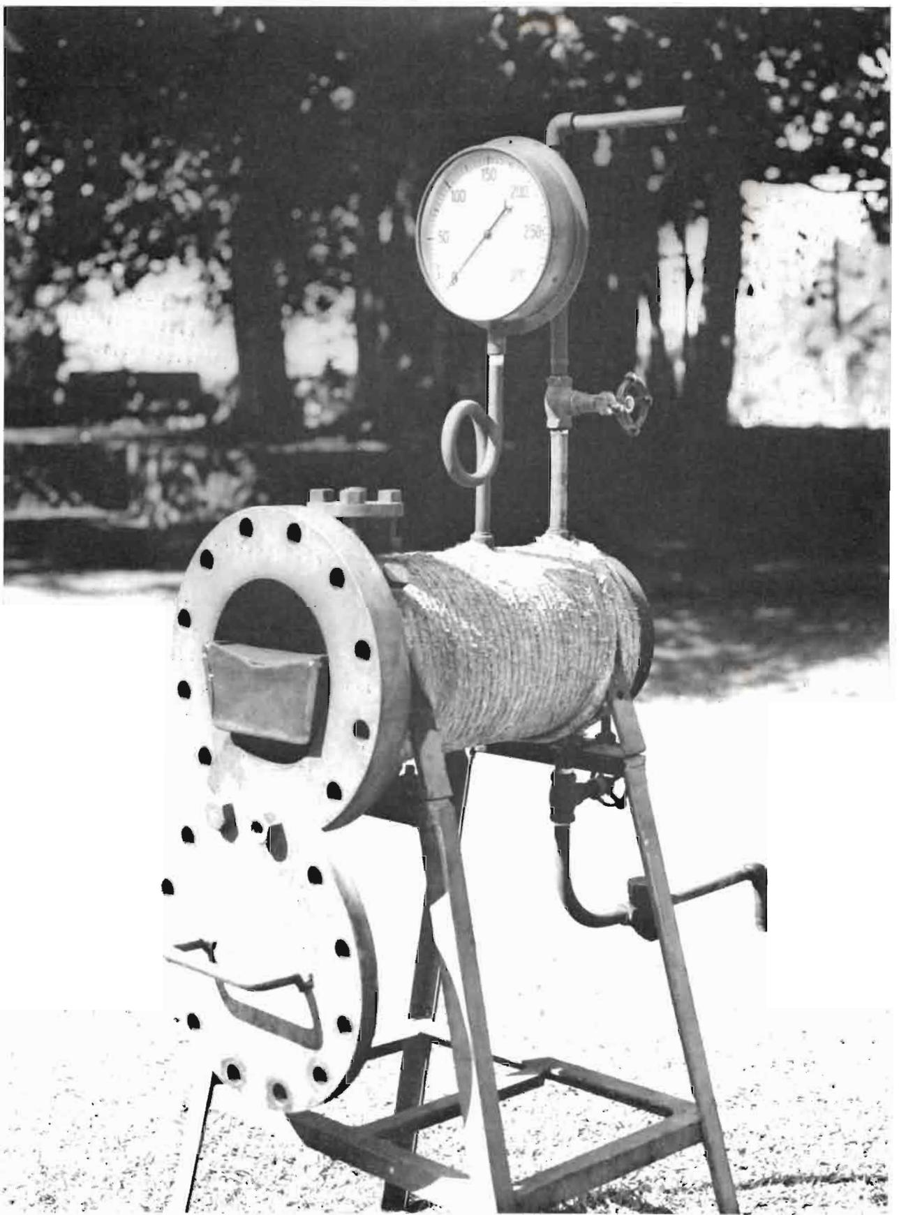
Plate VII. Digester used for steam treatment of bagasse (courtesy of Britannia S.E.)
