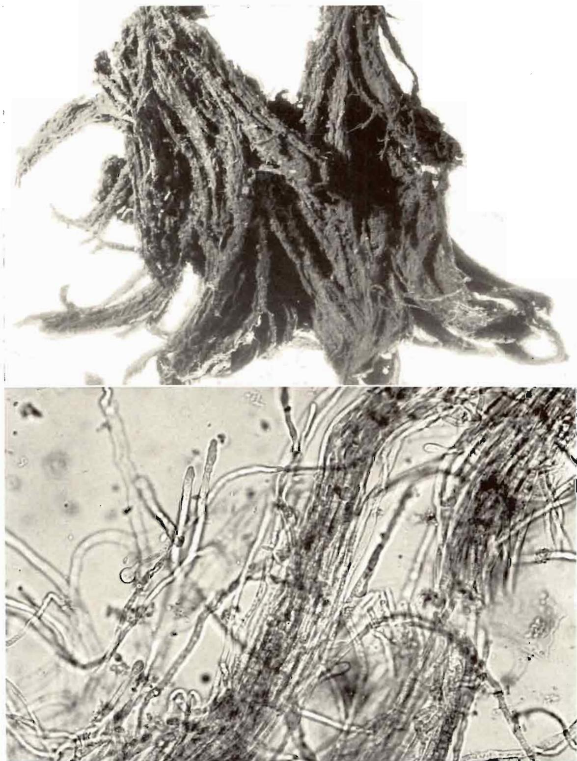
Micro-organism developing profusely in mixed juice tanks at a sugar factory.
