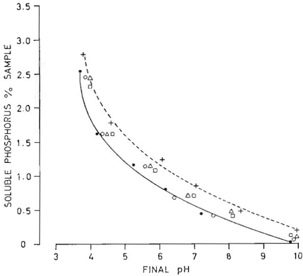
Fig. 11. Citrate solubility of guano at different particle sizes and pH levels.
