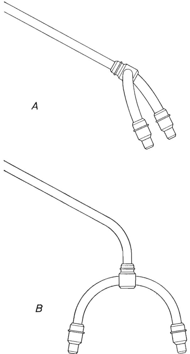
Fig. 31. A. Normal position of the nozzles on the handle-bar of the sprayer.
