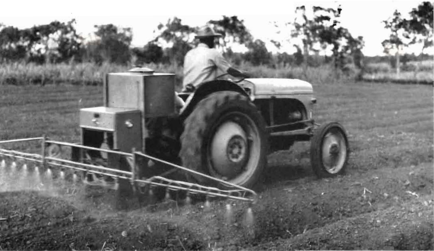
Screening of new herbicides with the Chesterford logarithmic spraying machine
