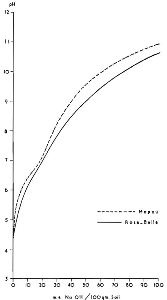
Fig. 14. Titration curves of two immature local soils.
