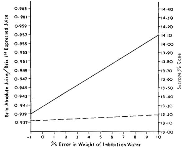
Fig. 30. Influence of weight of imbibition water on ratio  $B_A/B_1$  (plain line) and on sucrose content (broken line).
