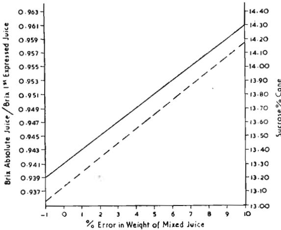
Fig. 29. Influence of weight of mixed juice on ratio  $B_A/B_1$  (plain line) and on sucrose content (broken line).
