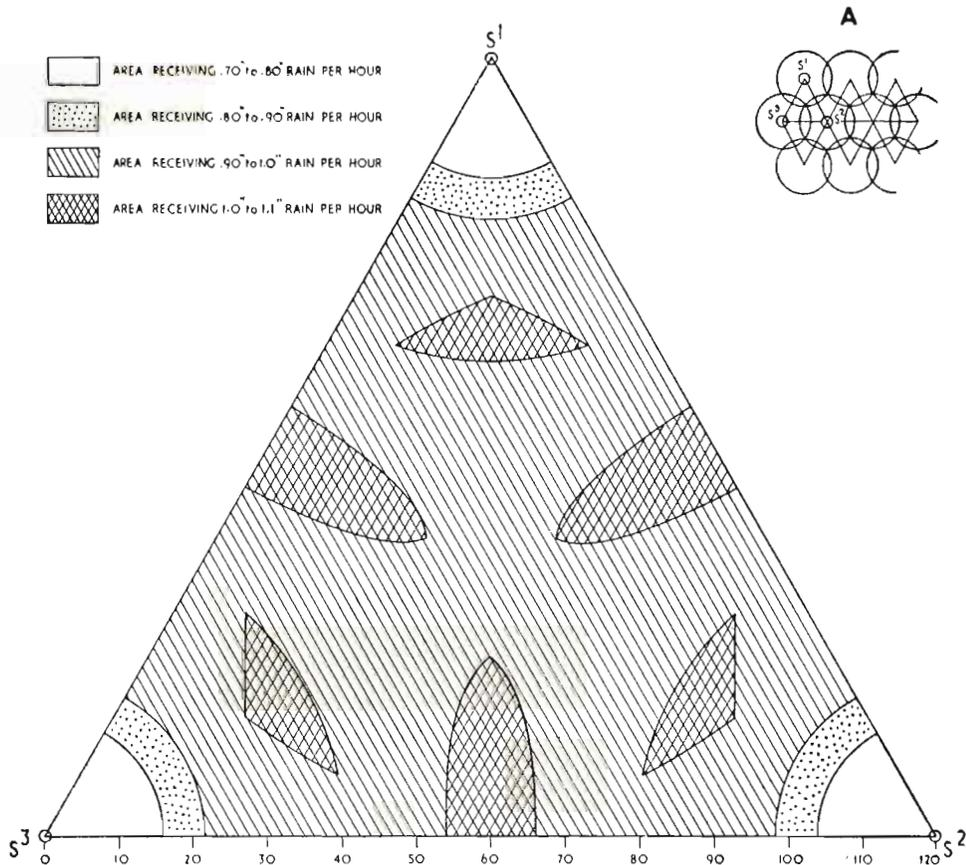
Fig. 27. Distribution of water from sprinklers S1, S2, S3 when arranged in the conventional pattern shown at A.
